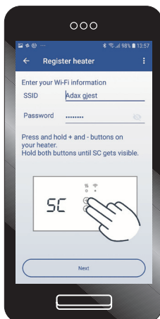
Register your heater and/or Smart Wi-Fi Plug. Follow the instructions given. Note! Your phone/device must be connected to the internet, through a Wi-Fi connection on your 2,4 GHz band. SSID/Network name must be your 2,4 GHz band.
